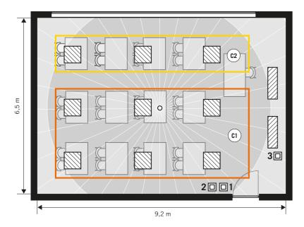
The lights close to the window and the lights further away from the window are assigned to separate light channels on the DUO DALI presence detector. This setting can also be overridden using the push button.
